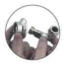
Carefully slide the dummy nuts onto the elbows ensuring damage to the plated surfaces is avoided.
