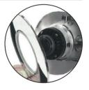
Fit the temperature lever and on/off control assembly to the valve body with the lever in a vertical position and the on/off control horizontal. Secure the assembly to the valve body with the four screws, hand tight only.
