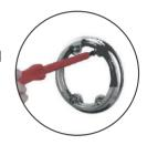
Insert the valve into the mounting ring and tighten the locking screw using the 2.5mm key provided.
